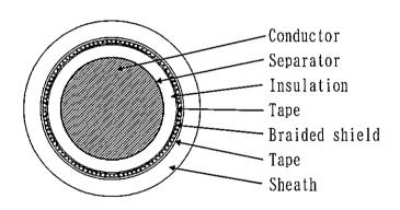
Fig. 1 Cable cross section
